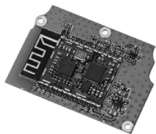
Built-in bluetooth module (inside the radio)
